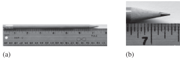
Figure 1.1 (a) Measuring the length of a pencil with a ruler. (b) Close-up view of the pencil tip.
